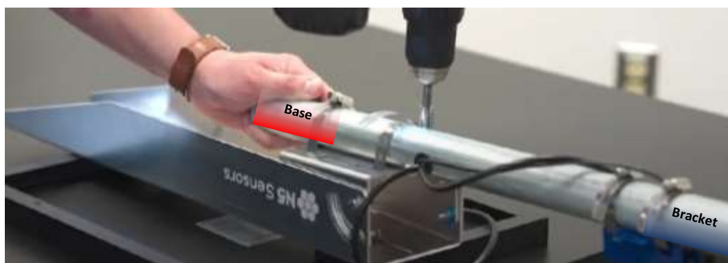
Figure 8: Solar pole connected to solar panel bracket
