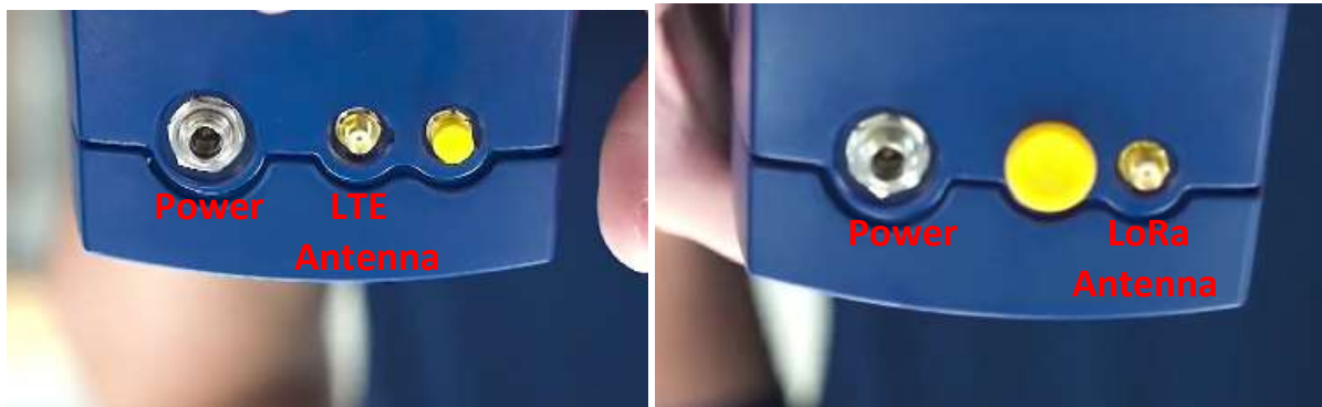
Figure 3: Power and Antenna connectors for LTE (Left) and LoRa (Right)
