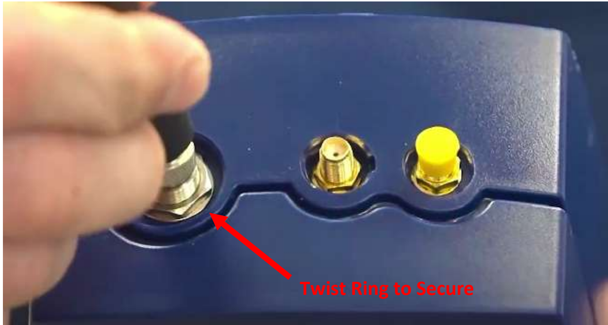
Figure 15: Insert and tighten threaded power connector onto ChemNode (LTE ChemNode Shown)
