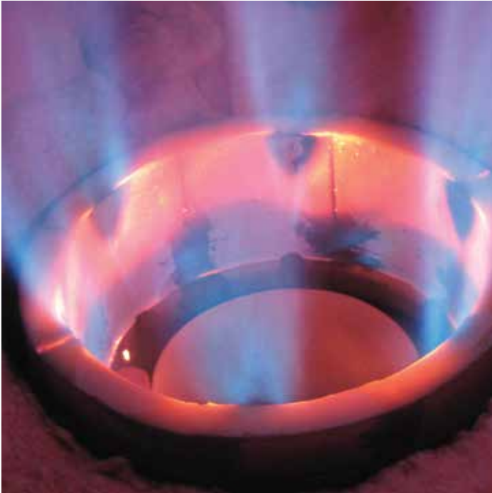
AK Staged Air Low-Emissions Combination Burner Operating on Gas Only
