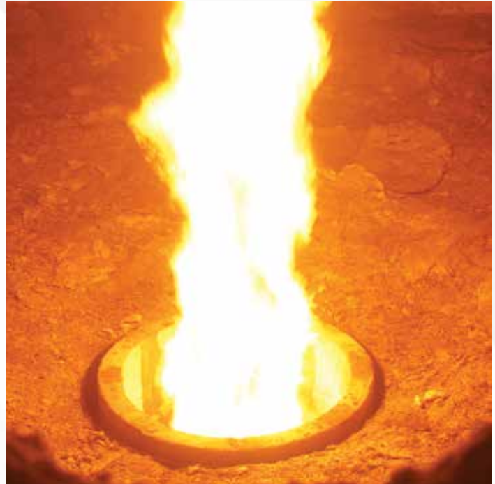
AK Staged Air Low-Emissions Combination Burner Operating on Oil Only
